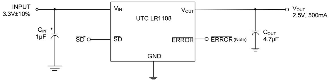
Note:  $\overline{SD}$  and  $\overline{ERROR}$  pins must be pulled high through a 10kΩ pull-up resistor. Connect the  $\overline{ERROR}$  pin to ground if this function is not used.
